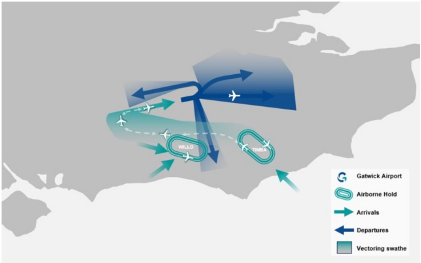
Figure 6: Simple illustration of the current Gatwick airspace and air traffic flows during easterly operations
